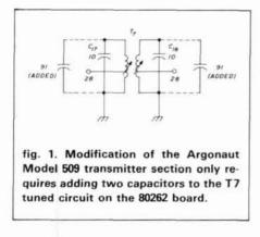
The Ten-Tec Argonaut 509 may easily be modified to cover 30 meters with the same performance found on its five bands. All that is required for the modification is five minutes of time, four components, and a jumper wire.
